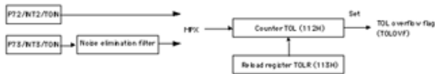
Figure 3.9 Block Diagram for Mode 1: 8-bit Reload Counter (T0L)
