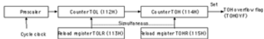
Figure 3.10 Block Diagram for Mode 2: 16-bit Reload Timer
